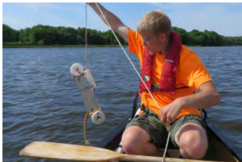
A staff member prepares to collect a water sample using a Van Dorn sampler.
