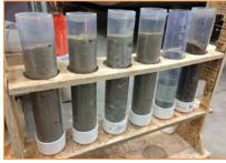
Figure 4-36 Spent Lime/Sand Mixture Column Testing
