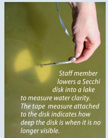
Staff member lowers a Secchi disk into a lake to measure water clarity. The tape measure attached to the disk indicates how deep the disk is when it is no longer visible.
