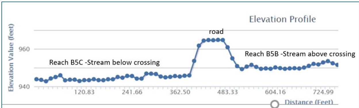
**Figure 4-9** LiDAR data for Bluff Creek streambed elevation showing elevation of stream bed for Reaches B5C and B5B.
