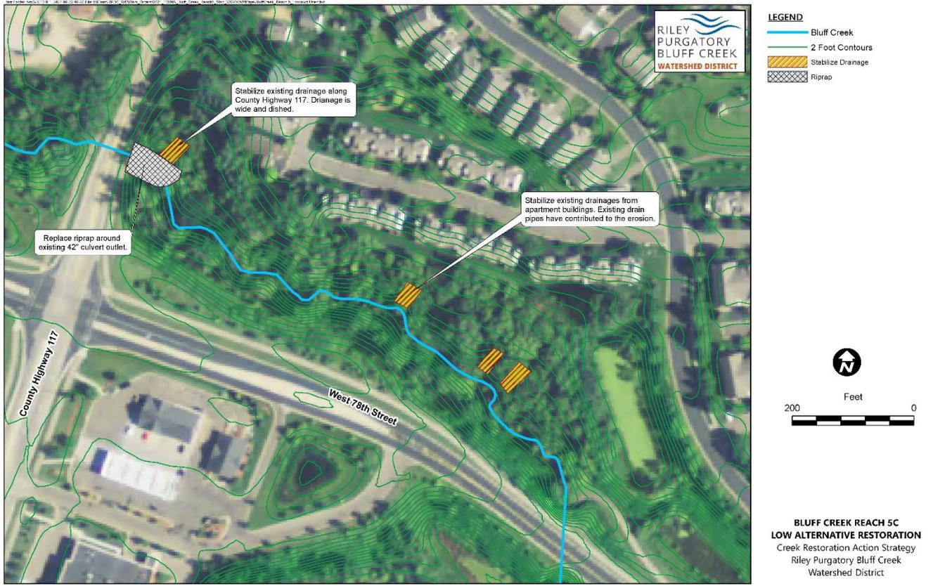
**Figure 5-5 Concept A: Low Concept Restoration of Reach B5C**
