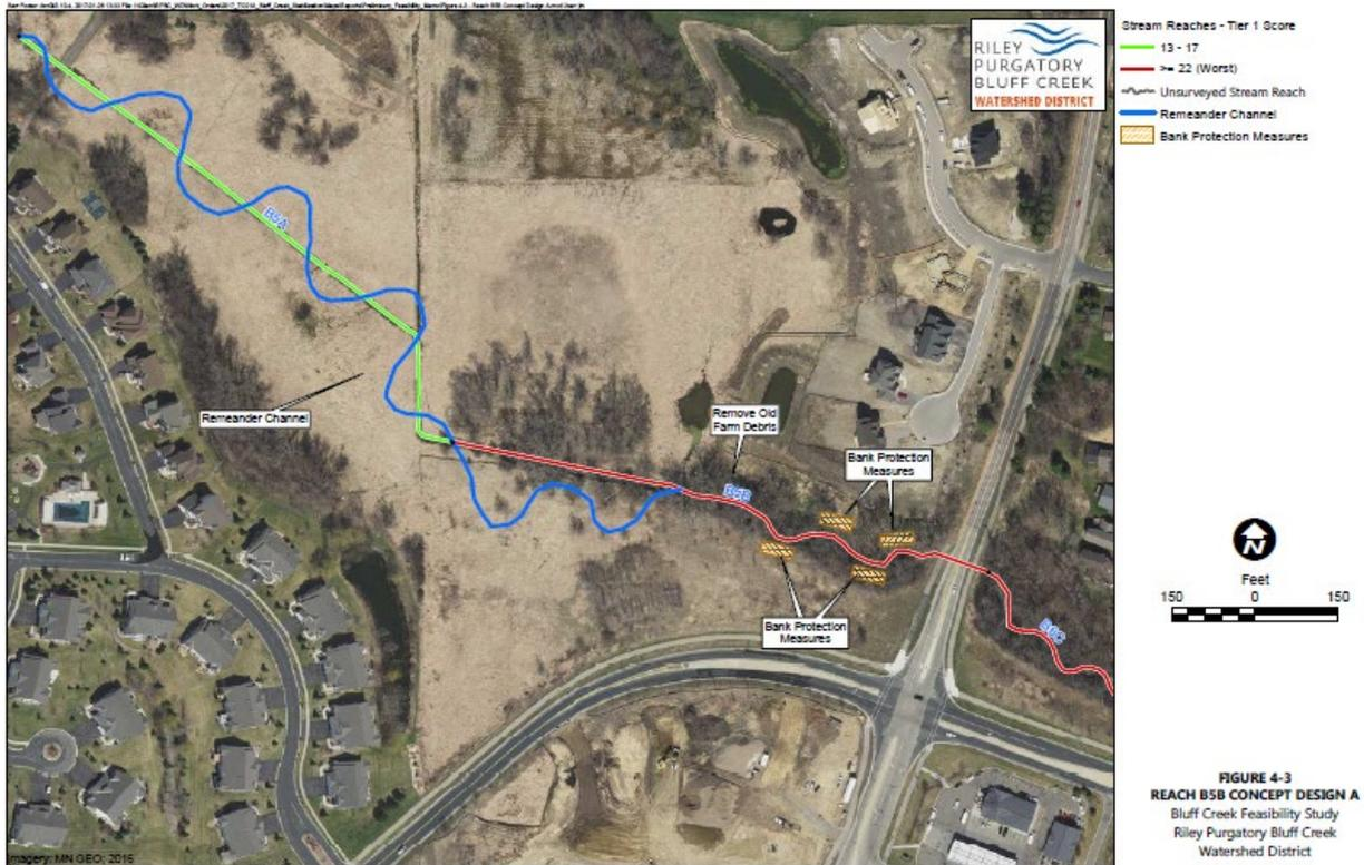
**Figure 5-3 Concept A: Restoration of Reach B5B by Remeandering**
