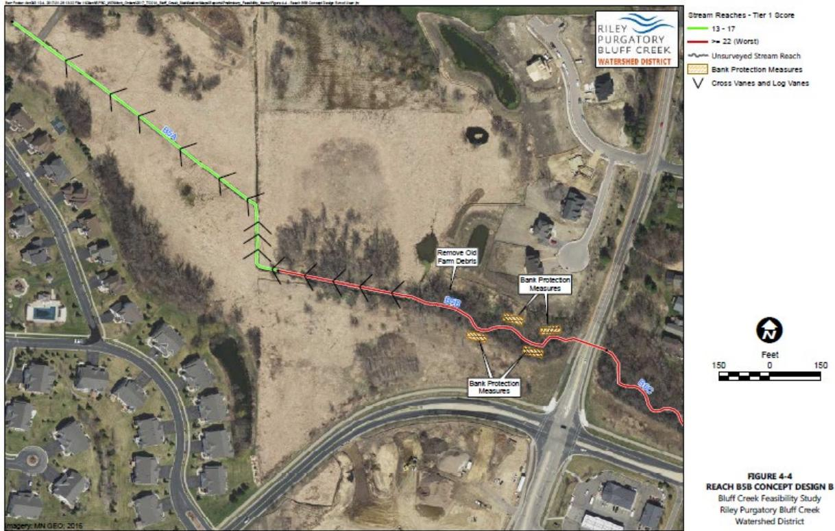
**Figure 5-4 Concept B: In-place Restoration of Reach B5B**
