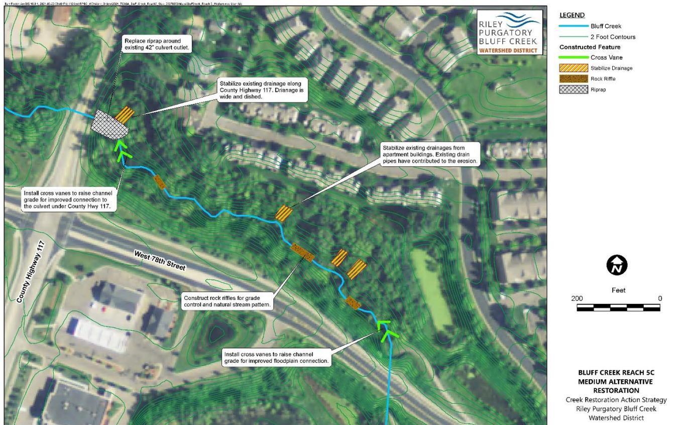
**Figure 5-8 Concept B: Moderate Concept Restoration of Reach B5C**
