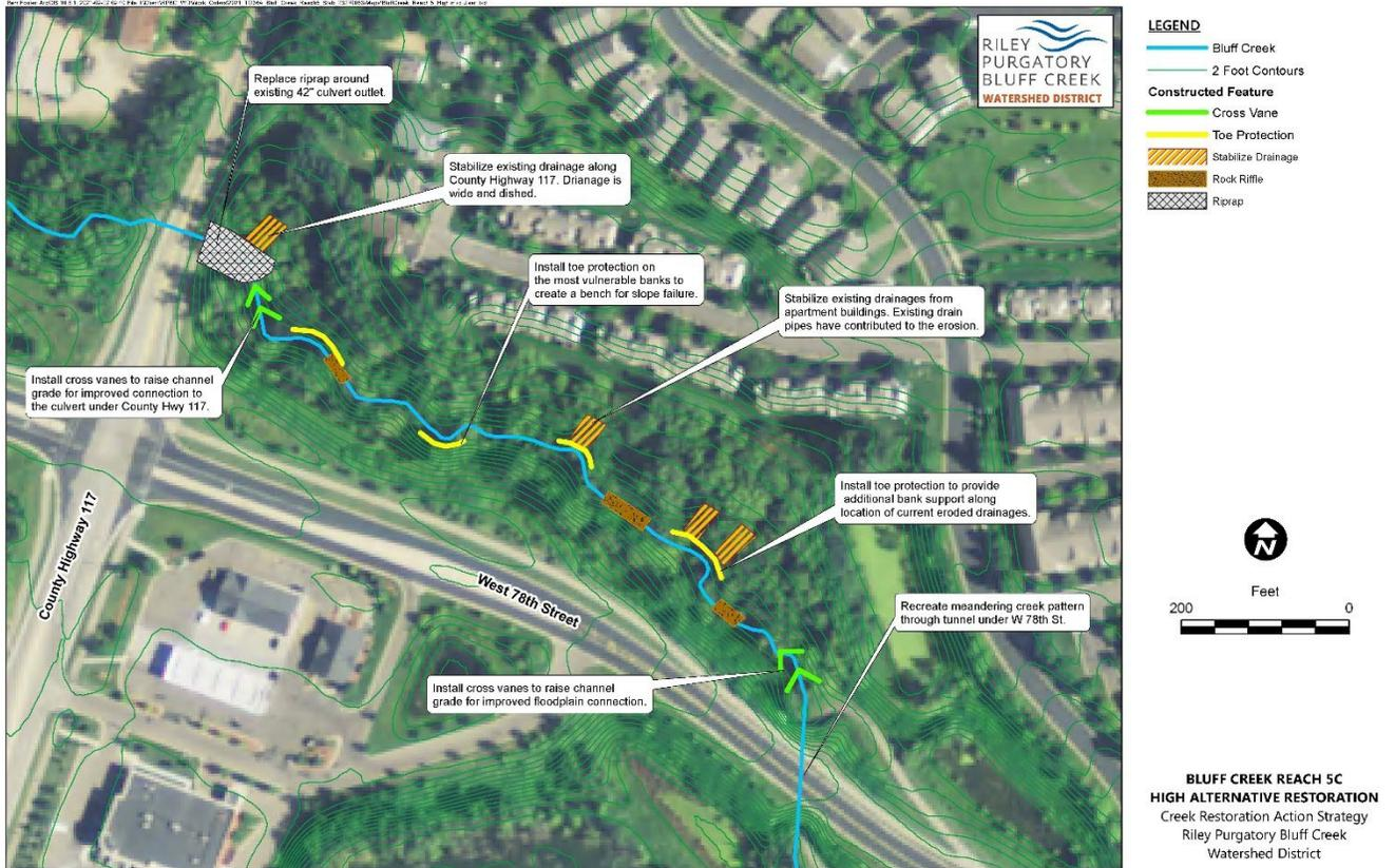
**Figure 5-9 Concept C: High Concept Restoration of Reach B5C**
