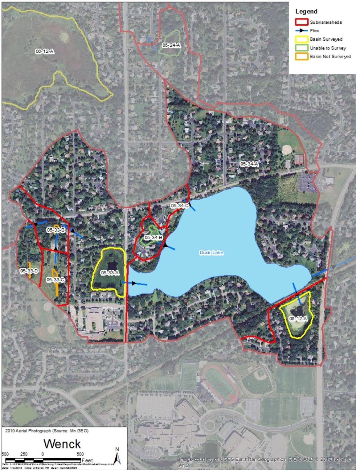
**Figure 3.2. Constructed Ponds, Wetlands and Flow Patterns in the Duck Lake Subwatershed.**
