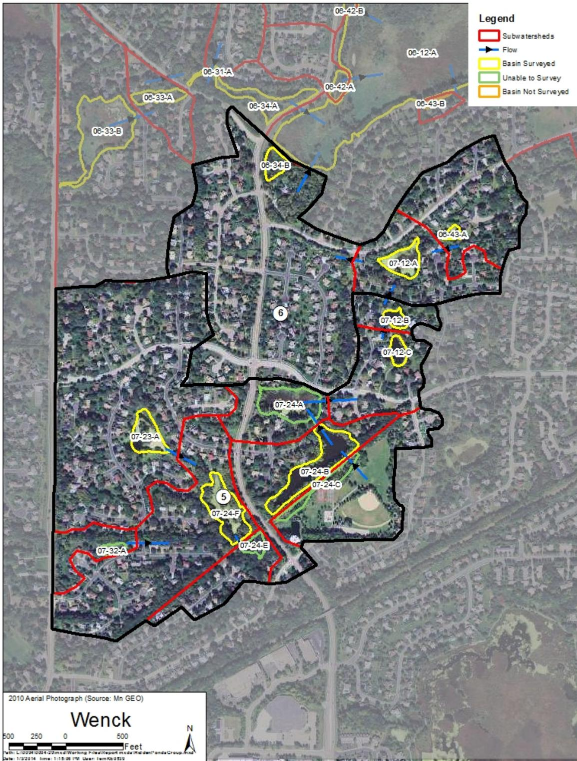
**Figure 3.5. Constructed Ponds, Wetlands and Flow Patterns in the Hidden Ponds Park Area Subwatershed.**
