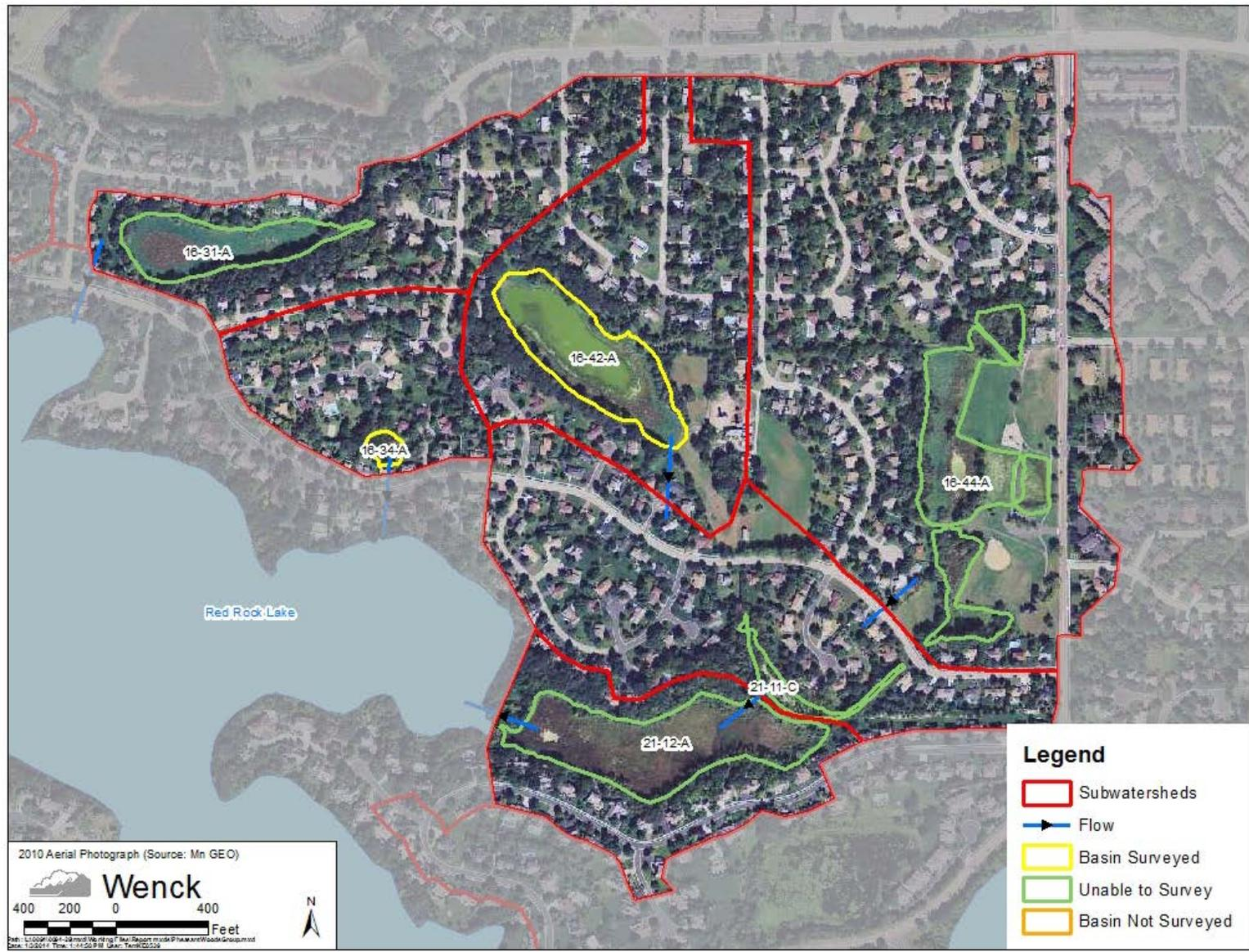
**Figure 3.9. Constructed Ponds, Wetlands and Flow Patterns in the Pheasant Woods Park Area Subwatershed.**
