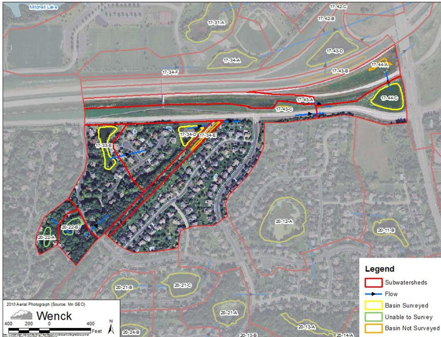
**Figure 3.7. Constructed Ponds, Wetlands and Flow Patterns in the Scenic Heights Road Area Subwatershed.**
