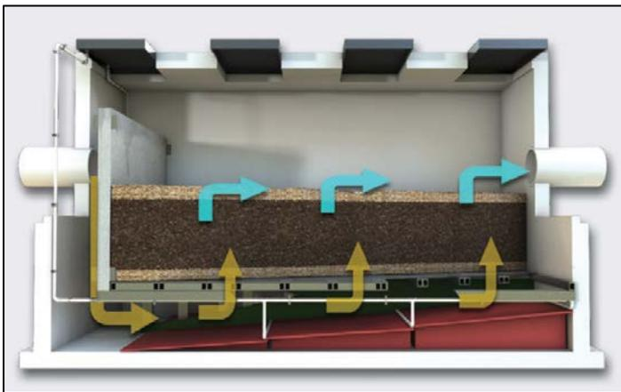
Schematic of the Nutrient Removing Filtration System® by SunTree (SunTree Technologies Inc., 2020).
