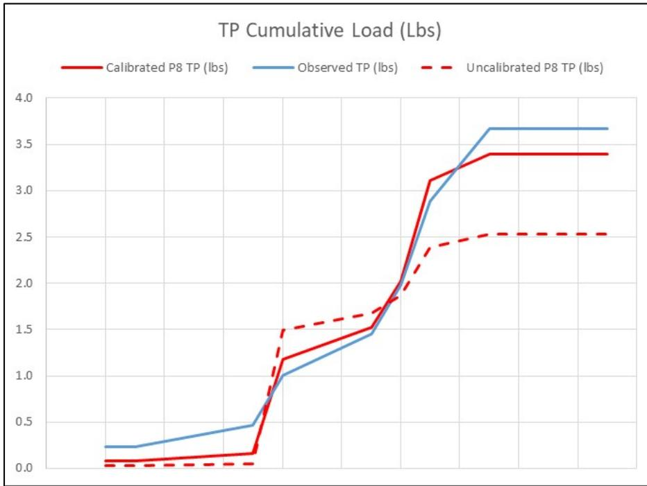
Figure 3-2 Modeled vs. Observed Cumulative Event TP Load
