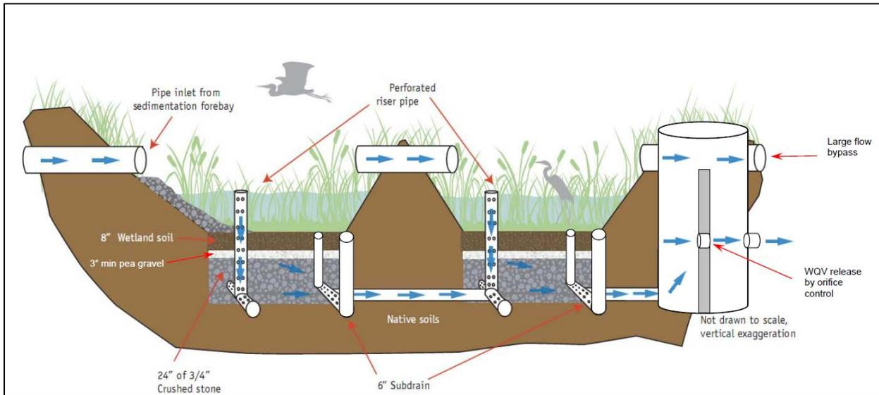
Schematic of a subsurface gravel bed wetland from the University of New Hampshire Stormwater Center Design Criteria (University of New Hampshire Stormwater Center (UNHSC), 2009).
