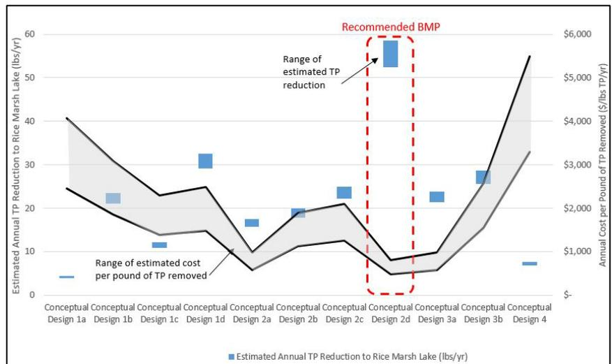
Of the eleven BMPs evaluated, the stand-alone Kraken Filter (or similar) has the lowest annualized cost per pound of phosphorus removed and greatest TP load reduction to Rice Marsh Lake.
