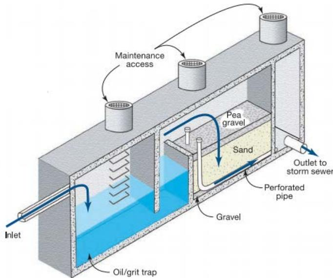
Example schematic of an underground sand filtration system (Protection, 2013).
