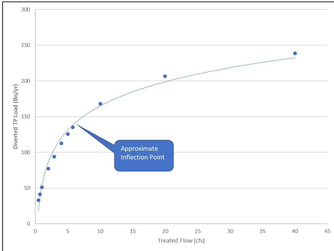
Figure 6-1 Estimated TP load to the potential BMP as a function of flow rate diverted to the BMP
