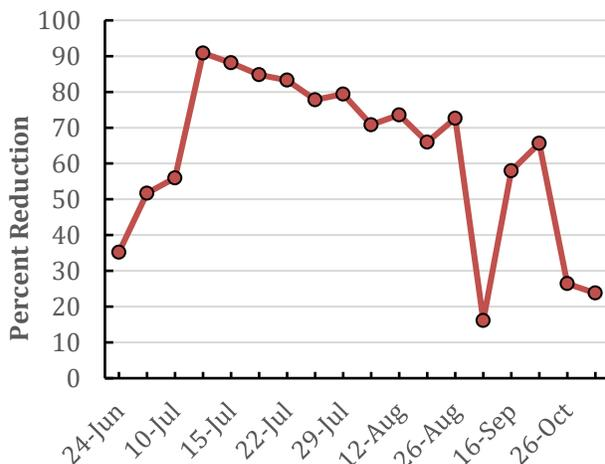
**Figure 4-39 2020 Lake Susan Spent Lime Treatment System Total Phosphorous Percent Reduction**
