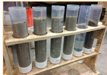
**Figure 4-36 Spent Lime/Sand Mixture Column Testing**
