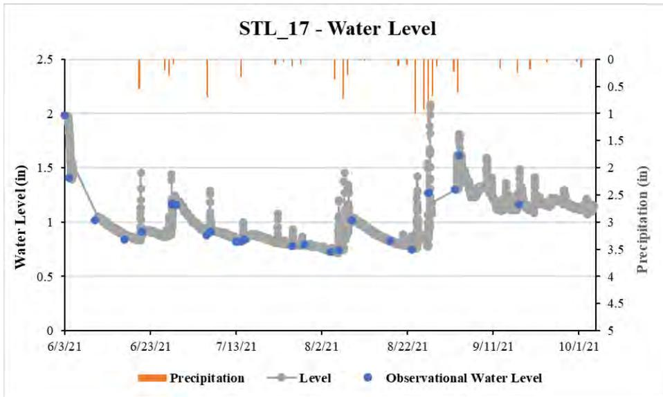
**Figure 4-23 Purgatory Creek/Staring Lake Road Water Levels**
