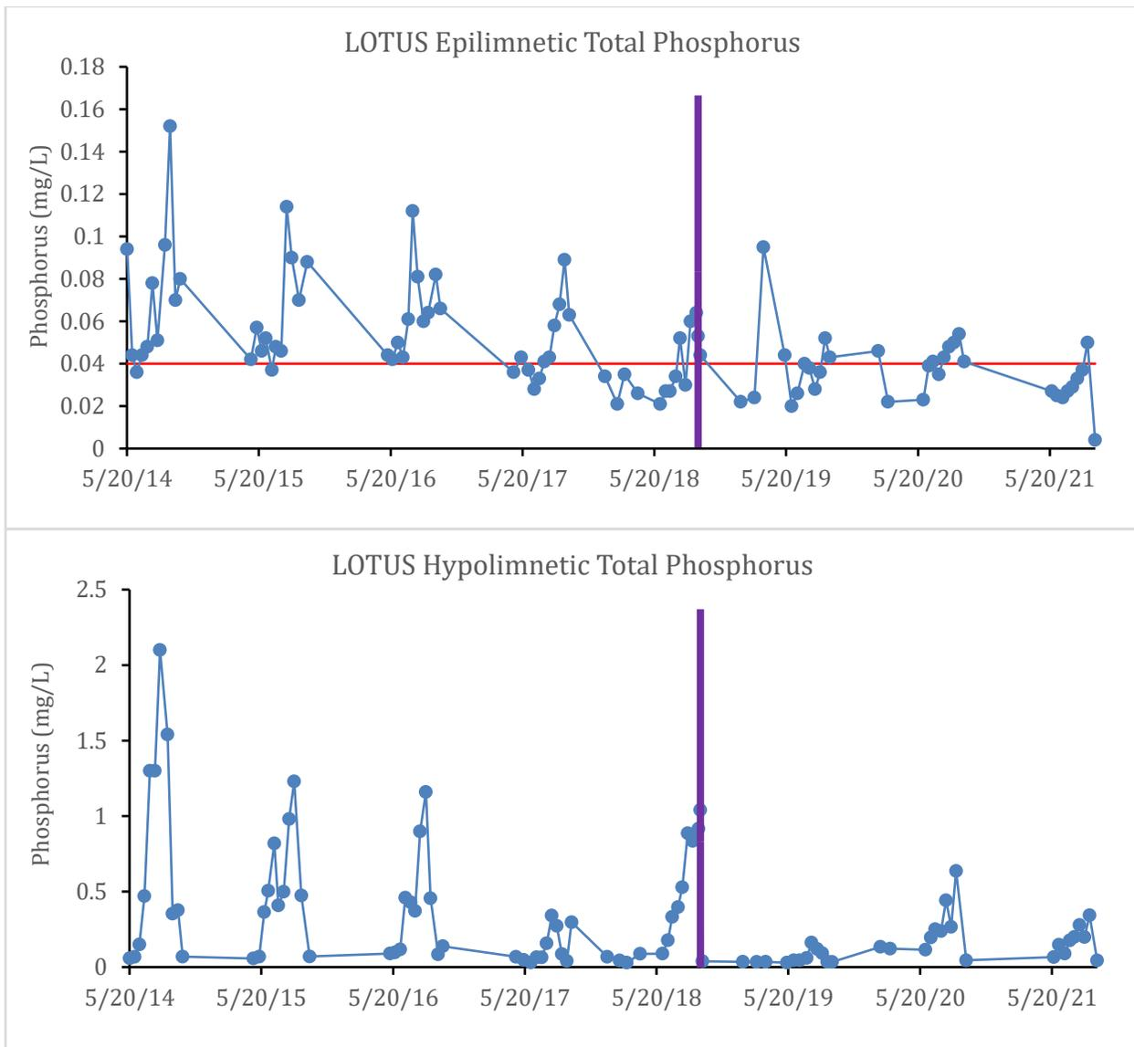
**Figure 4-7 Lotus Lake Total Phosphorus Levels pre- and post- Alum Treatment**
