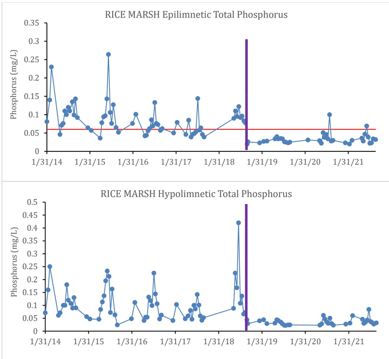
**Figure 4-6 Rice Marsh Lake Total Phosphorus Levels pre- and post- Alum Treatment**
